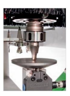
Reduction of tool change set-up time and the possibility of operator error, thanks to the contact pre-setter, which automatically determines the length of the tool.
