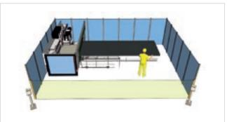
The machine can be configured with tandem loading in order to alternately process panels. This allows for loading or unloading to be carried out during machining operations.
