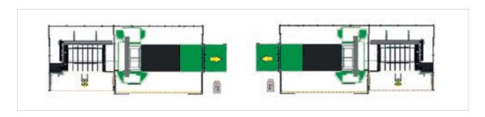
Loading/unloading operations are carried out simultaneously, allowing the operator to remove completed components from the unloading station in the utmost safety whist the machine is already processing the next panel.
