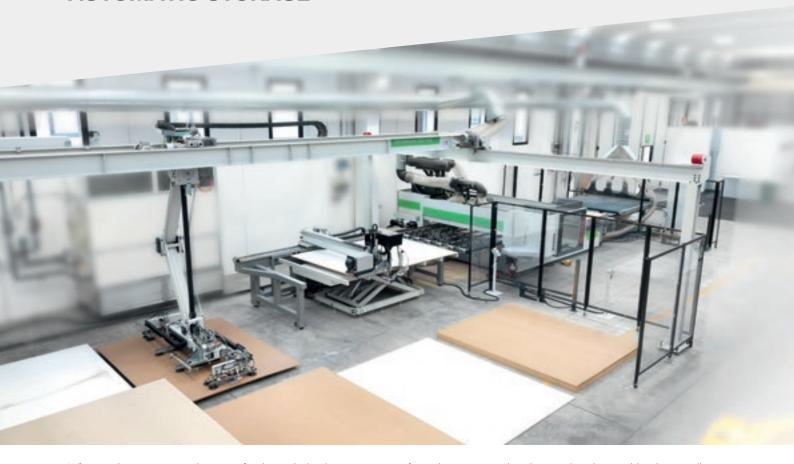
**Winstore** is an automated storage for the optimised management of panels. It ensures that the panels to be machined are easily accessible at all times, so it is possible to substantially increase cell productivity compared to manual loading methods using a forklift truck, without frequent stack changes.
