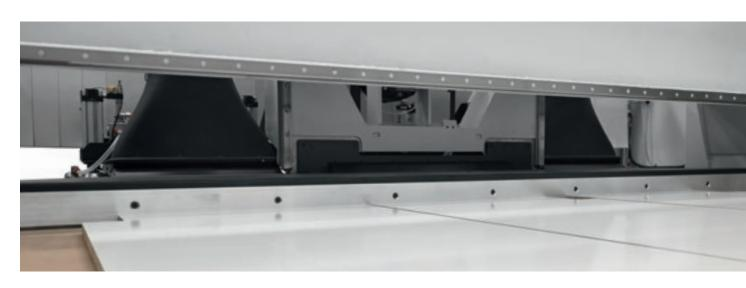
**Sweeping arm** with adjustable blade. Used to unload panels up to 3 mm thick.
