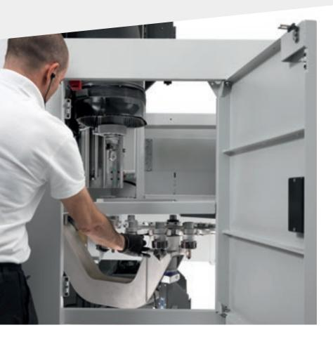
Tool change magazines with a total of up to 28 spaces. All tools and aggregates available at all times, with no need for operator intervention for tooling when switching from one machining operation to the next.
