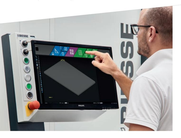
bTouch is the new 21.5" touch screen which enables you to carry out all of the functions previously performed using the mouse and the keyboard, enhancing the direct interaction between the user and the device.
